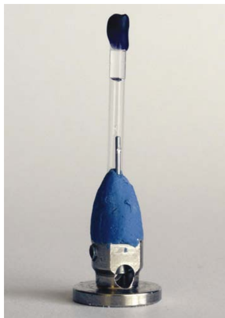
Figure 7 Loop-mounted crystal enclosed in a quartz capillary. The column of mother liquor used to stop the crystal drying out can be seen at the top of the capillary.
